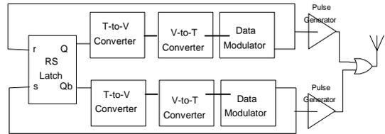
**Figure 4:** Top level of transmitter design, showing multiplexed parallel architecture
