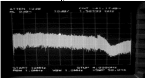
**Figure 9:** Power Spectral Density of Chaotic Pulses of Time Duration < 1ns
