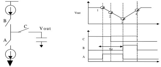
**Figure 3:** Voltage-to-Time Converter: Charge Pump Behavior and Tent Map Example
