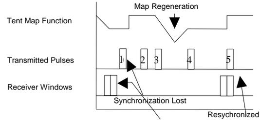
**Figure 6:** Example of receiver losing lock and regaining synchronization
