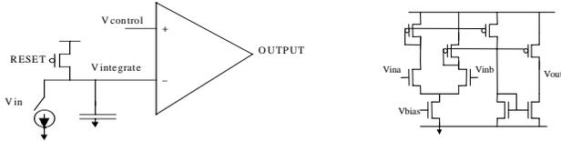
**Figure 2:** Time-to-Voltage Converter, with Opamp Schematic
