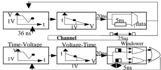
Figure 1: Top Level Diagram of Chaotic Transmitter and Drive-Response Receiver
