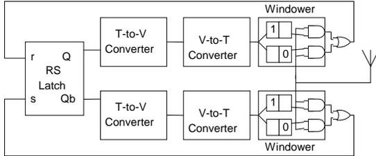
**Figure 5:** Top level of receiver design, showing operation of windowing block
