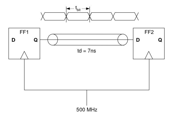
The data travels on the link from FF1 to FF2. The delay of the wire is  $t_{wire} = 7ns$ .
