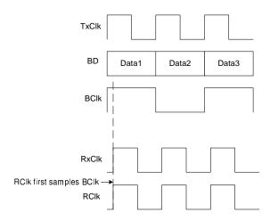
Since BClk is high, the RC filter, acting as an integrator, will increase the delay between RxClk and RClk by an amount,  $t_{del\,ay}$ , as noted in the diagram below.
