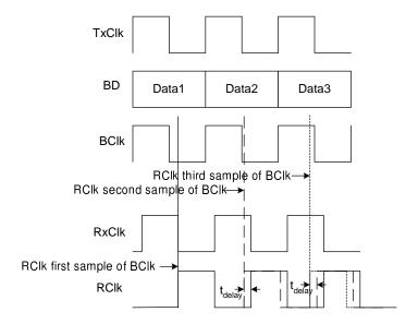
Upon the first sample, RClk samples BClk as low. This decreases the delay of RClk with respect to RxClk by an amount  $t_{delay}$ . This RClk, that has a smaller delay from RxClk than before, is shown in the dashed lines.
